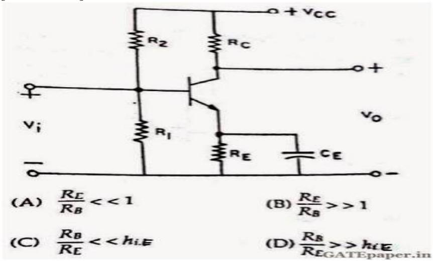
5. Which of the following statements are correct for biasing transistor amplifier configurations? [GATE 1990] [ ]
