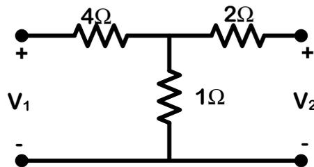
9. a) The given ABCD parameters are  $A=2$ ,  $B=0.9$ ,  $C=1.2$ ,  $D=0.5$ . Find Y-parameters. [L3][CO2][5M]
