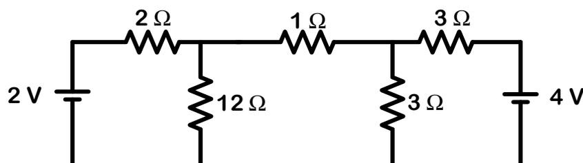
6. Find the current delivered by the source for the circuit shown in figure. [L3,CO1,10M]
