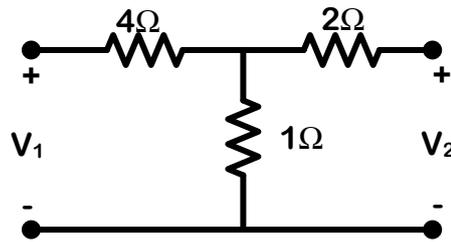
8. Find the Short circuit parameters for the given circuit. [L4][CO2][10M]
