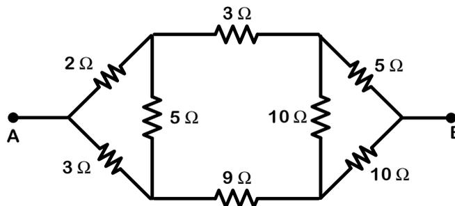
8. Explain in detail about star to delta transformation of given resistive network. [L2, CO1,10M]
