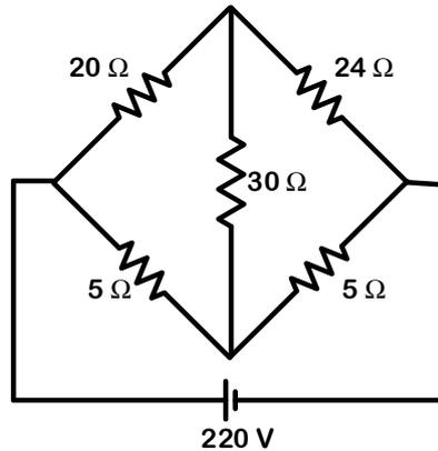
7. Find the voltage to be applied across AB in order to drive a current of 5A into the circuit. [L5,CO1,10M]
